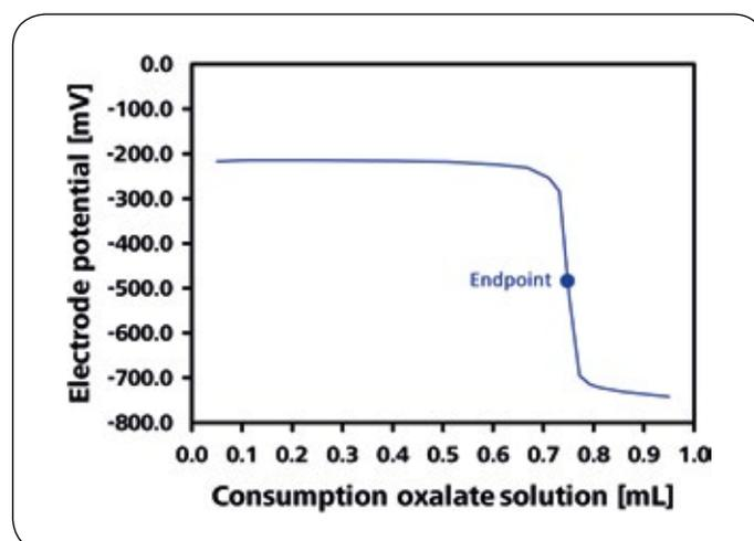
Fig. 2: Titrimetric determination of the permanganate index: consumption of oxalate volume versus measured electrode potential
