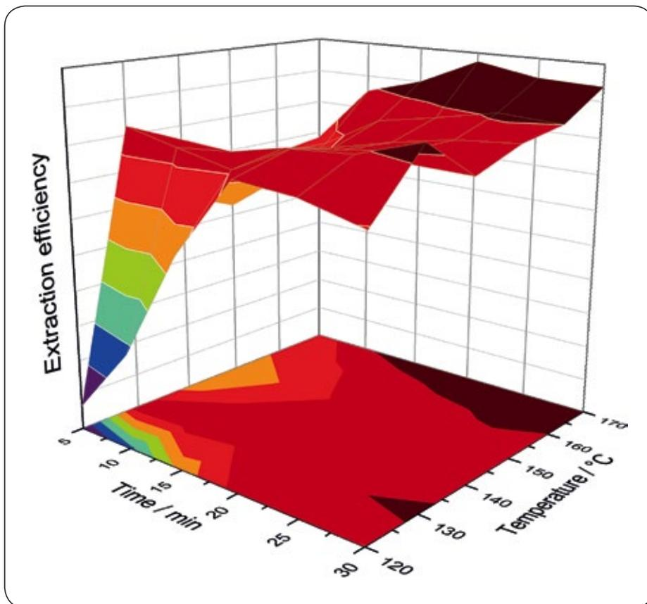
Fig. 2: Optimization of the extraction procedure for Irganox 1330 in polypropylene extracted with ethyl acetate
