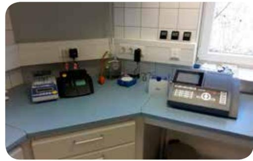
Fig. 3: photoLab 7600 UV-VIS photometer for the measurement of optical, reagent-free (OptRF) methods in the laboratory of the WWTP Peißenberg
