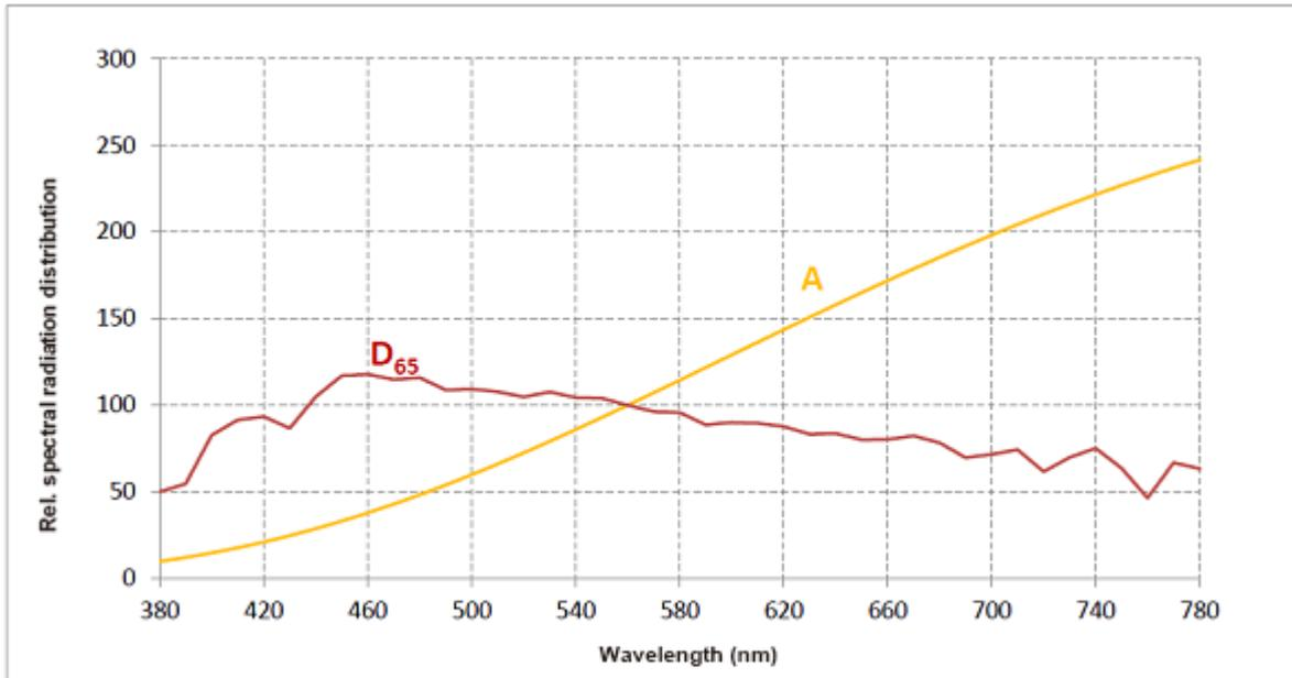
**Fig. 2** Relative spectral radiation distribution of the standard illuminants A and D<sub>65</sub>
