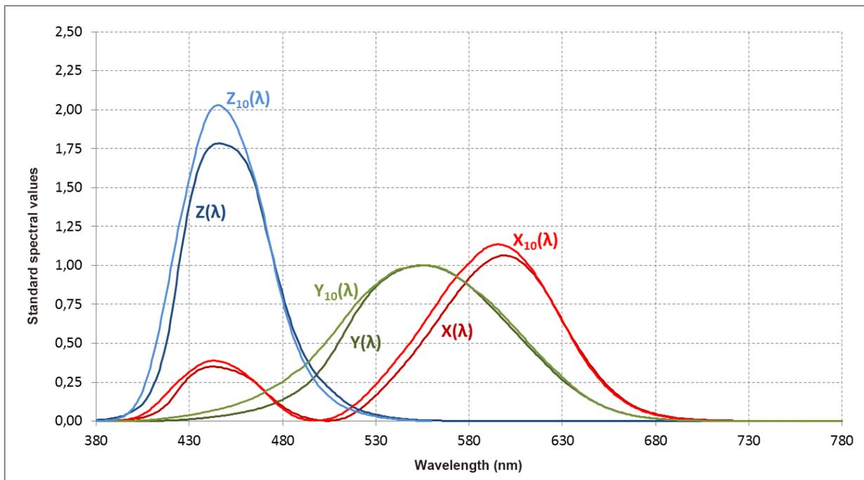
**Fig. 1** Standard color matching functions for 2° and 10° observers.
