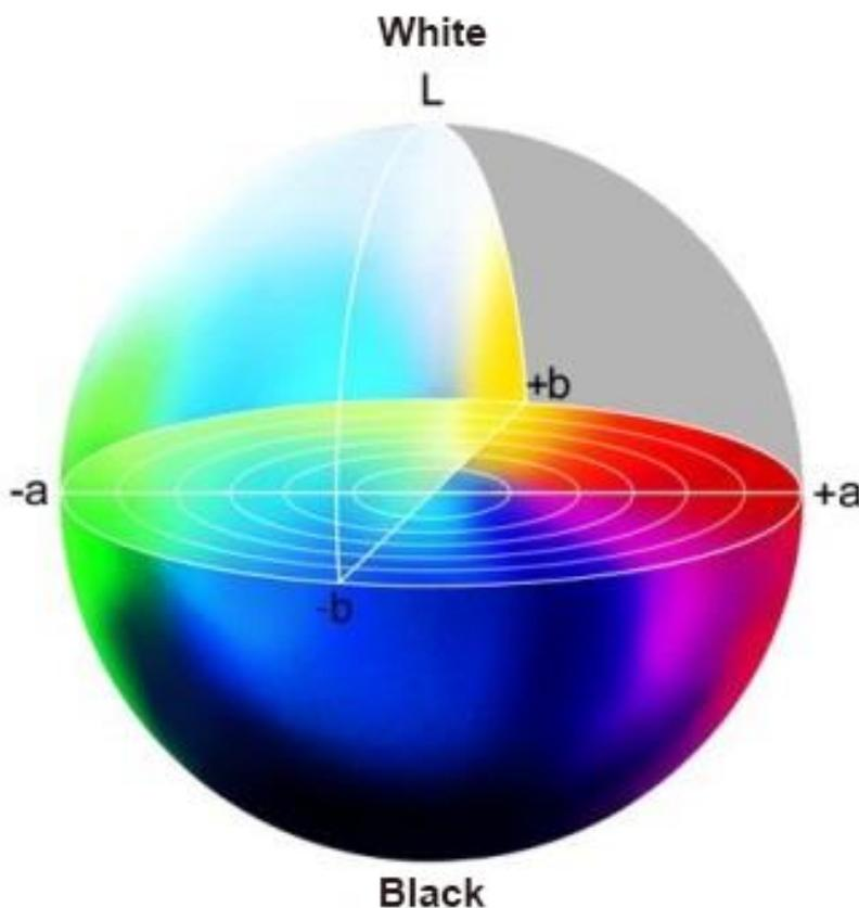
*Fig. 4: Diagram of the three-dimensional CIE-L\*a\*b color space*
