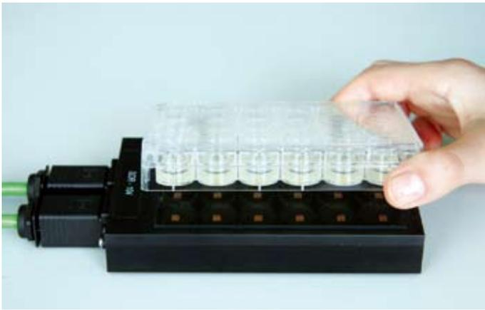
Fig. 1: SDR SensorDish Reader for on-line monitoring of dissolved oxygen and pH in 24-well multidishes.
