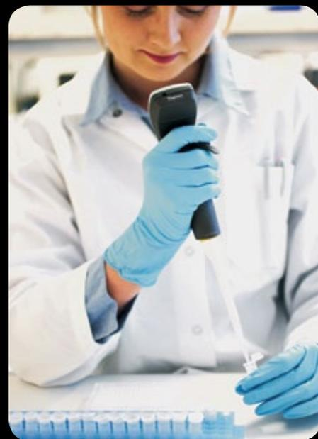
Utilizing index finger trigger action, shown here with the Thermo Scientific FinnpiPETTE Novus, significantly reduces risk of injury.
